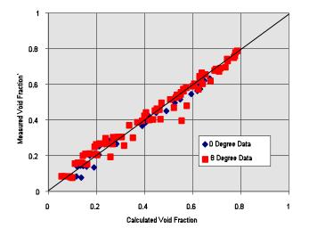
The fit in the countercurrent quadrant (away from the countercurrent flow limit) is quite good and provides a significant improvement over the previous engineering approximation.
