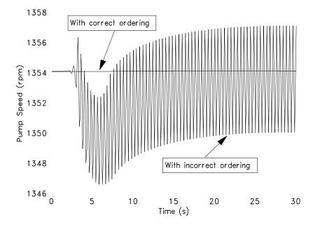
Figure 1. Illustration of the Effect of Control Block Ordering
